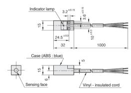
Note; Vinyl-insulated cord (oil-resistant: 0.3mm², 27/0.12 dia., 3-core) 4.2mm dia.
