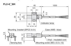
Note; A mounting bracket and two mounting screws and provided. Vinyl-insulated cord (oil-resistant: 0.3mm², 27/0.12 dia., 3-core) 4.2mm dia.
