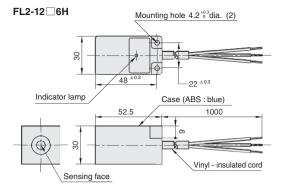
Note; Vinyl-insulated cord (oil-resistant: 0.3mm², 20/0.18 dia., 3-core) 5.7mm dia.
