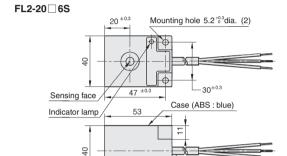
Note; Vinyl-insulated cord (oil-resistant: 0.5mm², 20/0.18 dia., 3-core) 5.7mm dia.
