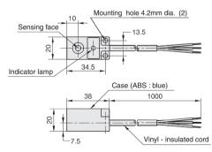
Note; Vinyl-insulated cord (oil-resistant:  $0.3 mm^2$ , 27/0.12 dia., 3-core) 4.2 mm dia.
