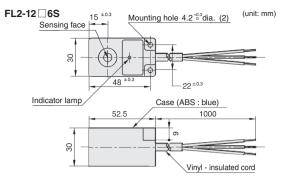
Note; Vinyl-insulated cord (oil-resistant: 0.3mm², 20/0.18 dia., 3-core) 5.7mm dia.
