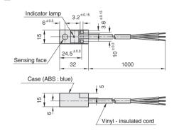
Note; Vinyl-insulated cord (oil-resistant:  $0.3 mm^2$ , 27/0.12 dia., 3-core) 4.2 mm dia.
