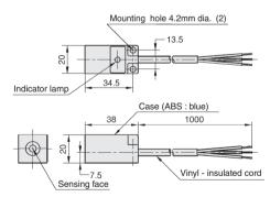
Note; Vinyl-insulated cord (oil-resistant: 0.3mm², 27/0.12 dia., 3-core) 4.2mm dia.
