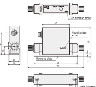
Hole for attaching mounting plate: φ 5.6
