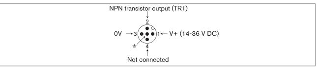
Fig. 17 : Pin assignment of the male fixed connector on a version with 1 NPN transistor output and 1 current output
