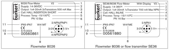
Fig. 1 : Examples of a name plate
