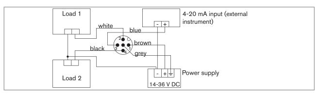
Fig. 26 : PNP wiring of both transistor outputs and wiring the current output in sourcing mode (parameter setting "PNP/ source"), of a version with 1 M12 fixed connector
