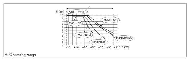
Fig. 3 : Fluid temperature-pressure dependency for the flowmeter 8026 associated to a fitting S020
