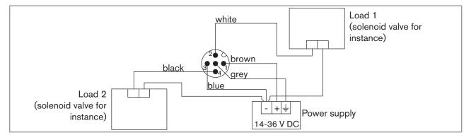
Fig. 23 : PNP wiring of both transistor outputs (parameter setting "PNP/source"), of a version with 1 M12 fixed connector
