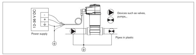
Fig. 16 : Equipotentiality skeleton diagram with pipes in plastic
