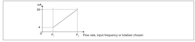
*Fig.* 38 : 4-20 mA current according to the chosen physical parameter or totalizer
