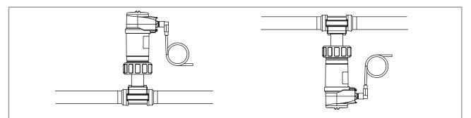
Fig. 9 : The paddle wheel axis must be horizontal
