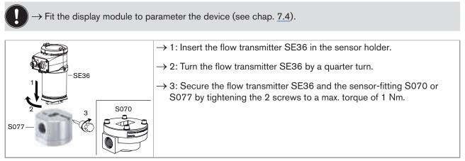
Fig. 13 : Assembling the flow transmitter SE36 with sensor-fitting S070 or S077
