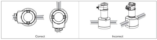
Fig. 12 : The oval gear axes must be horizontal
