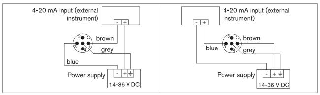
*Fig.* 19 : Possible electrical connections of the current output only, on a version with 1 M12 fixed connector, 1 NPN transistor output and 1 current output
