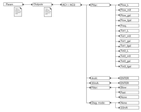
Functions "4mA" and "20mA" are used to define the measurement range for the flow rate, the input frequency or the totalizer associated with the current on the 4-20 mA output.
