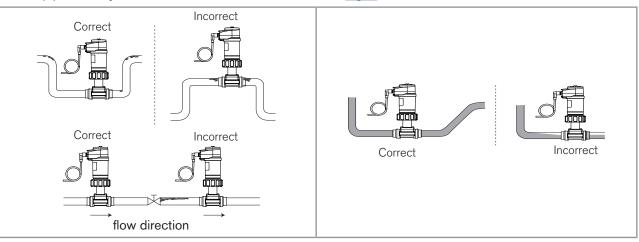
Fig. 8 : Air bubbles within the pipe / Filling of the pipe
