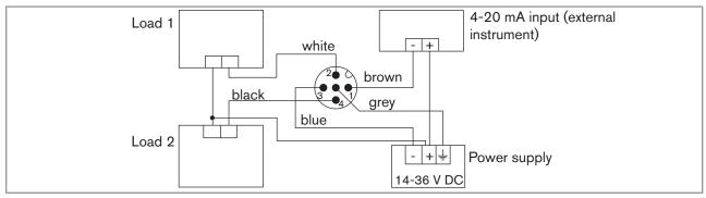
Fig. 25 : NPN wiring of both transistor outputs and wiring the current output in sinking mode (parameter setting "NPN/ sink"), of a version with 1 M12 fixed connector
