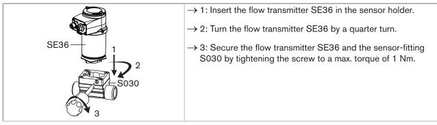
*Fig.* 11 : Assembling the flowmeter 8036
