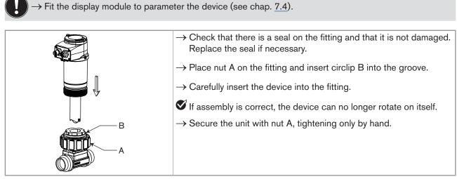
Fig. 10 : Installation of flowmeter 8026 into the fitting S020
