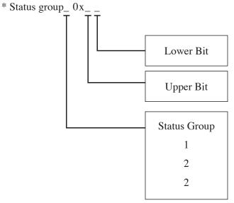
"Status Group 0 0xC3" of the diagnostic result is as follows. The codes "C" and "3" are in accordance with the following tables.
