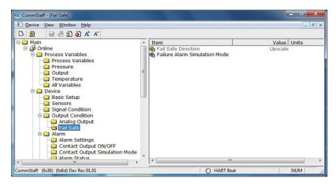
Failure Alarm Simulation Mode allows you to perform a simulation of output current in abnormal operating conditions.
