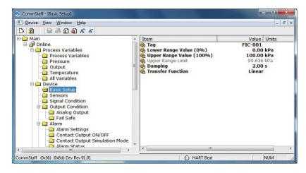
Linear: Linear output Sq root: Square root output
