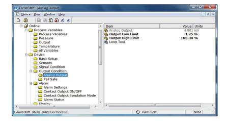
Select Device  $\rightarrow$  Output Condition  $\rightarrow$  Analog Output.
