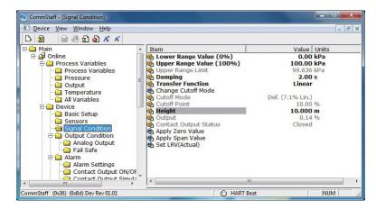
Input the height difference between the flanges in meters. If this function is not enabled, "0.00 m" is displayed.
