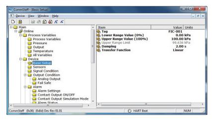
Lower Range Value (0%): Value at which 4 mA is output Upper Range Value (100%): Value at which 20 mA is output
