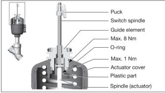
Fig. 13: Installing the switch spindle (2), external pilot air duct
