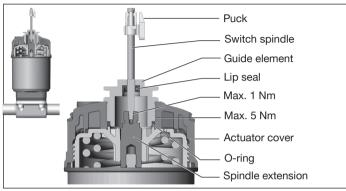
Fig. 8: Installing the switch spindle (2), integrated pilot air duct
