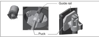
Fig. 10: Aligning the puck
