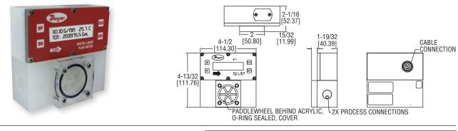
The SERIES DPW Digital Paddlewheel is an economical choice for applications where remote or local liquid flow measurement is desired. This Series offers two programmable totalizers via the optional LCD and RS-232/RS-485 interface, two optically isolated flow pulse outputs, and selectable 0 to 5 VDC or 4 to 20 mA flow outputs (optional temperature).
