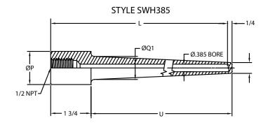
(\*) Thermowells with an overall length of 42" or less are machined from SOLID BAR STOCK. Thermowells with an overall length greater than 42" are constructed using a welded design and are available in straight, stepped or tapered design. However, for tapered only the last 16" are tapered.
