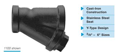
The Trerice **1100 Series** Pipeline Strainer is designed to be installed upstream of regulators, valves, or other similar equipment. This Y-Type Strainer removes debris from the line, thereby providing protection and extending the life of the regulator or valve. The 1100 Series has a generously proportioned, cast-iron body and a  $1/_{64}$ " perforated, stainless steel screen. A blow-out valve should be installed so that the screen may be cleaned periodically.
