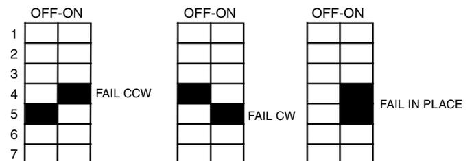
**Note: DIP #4 & DIP #5 are not active when input jumper is on 10V / SW**
