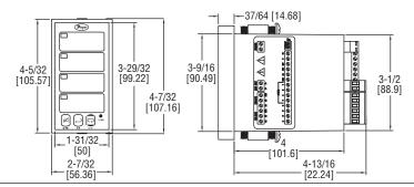
The **SERIES AN2** Indicating Alarm Annunciator provides visible and audible alarms for up to eight inputs. Audible alarm conditions can be acknowledged, reset, or silenced either via the front panel push buttons or the rear terminal block. The annunciator also has two SPDT relay outputs that can be used to initiate external alarms, buzzers, or paging devices.
