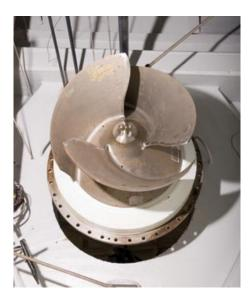
This Flowserve high-quality impeller is cast and machined to tight tolerances to ensure high efficiency and performance.
