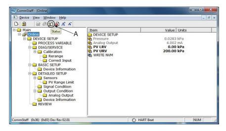
For example, the button to the left of CORRECTS RESET turns red after the calibrated values are reset.
