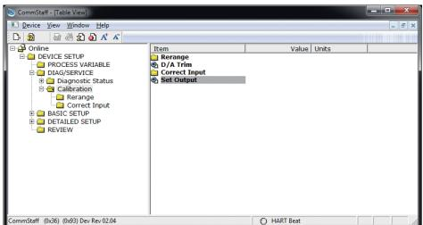
•  $[DEVICE SETUP] \rightarrow [DIAG/SERVICE] \rightarrow [Calibration] \rightarrow [Set Output]$
