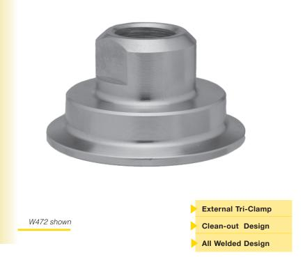
The Trerice **Sanitary Diaphragm Seal** is intended for use in the food and pharmaceutical industries, or in any application where a thorough cleaning of the wetted surface is required. Ease of maintenance is ensured as surfaces that contact the process media are virtually free of crevices. The all welded construction and external Tri-Clamp connection allow for easy removal and cleaning.
