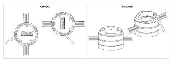
The pipe must be filled with liquid and free from air bubbles. Avoid air purge of the system which would cause damages and to prevent damage from dirt or foreign matter, we strongly recommend the installation of a 250  $\mu$ m strainer as close as possible to the inlet side of the meter.
