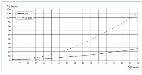
The diagram shows exemplarily the pressure loss characteristics when air flowing through. For determining the pressure loss with another gas it needs to calculate the air equivalent and respect the fluidics needed with the other gas.
