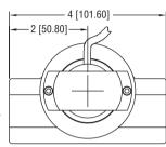
The **SERIES SFI-100T** Sight Flow Indicators & Transmitters is a low cost and durable flow transmitter that combines our popular 100 Series Sight Flow Indicator with our A-711T output sensor for visual and remote monitoring of flow. The A-711T output sensor has two pulsed voltage signals with one providing a 5 VDC pulse, the other a pulse of the input supply voltage used, ranging from 8 to 28 VDC and a pulsed output with a frequency change proportional to the flow rate.
