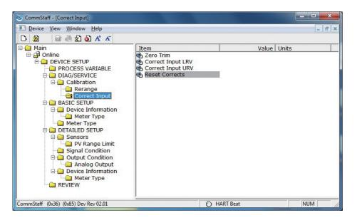
CAUTION: If this operation is performed while the pressure transmitter process is under automatic control, outputs may fluctuate, making pressure transmitter operation dangerous. Before performing this operation, make sure that you switch the process control loop to manual control.
