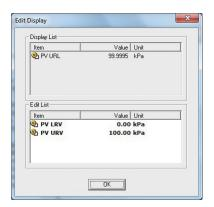
LRV: Value at which 4 mA is output URV: Value at which 20 mA is output
