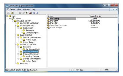
If SFN communication is used, set a value in the range of 0 to 32 seconds.
