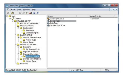
Double-clicking Loop Test displays the following screen.
