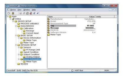
Double-clicking Tag displays the settings screen. On this screen, set the Tag and click the Set button. The tag is highlighted in yellow. Click the Send button to send the new Tag to the pressure transmitter.
