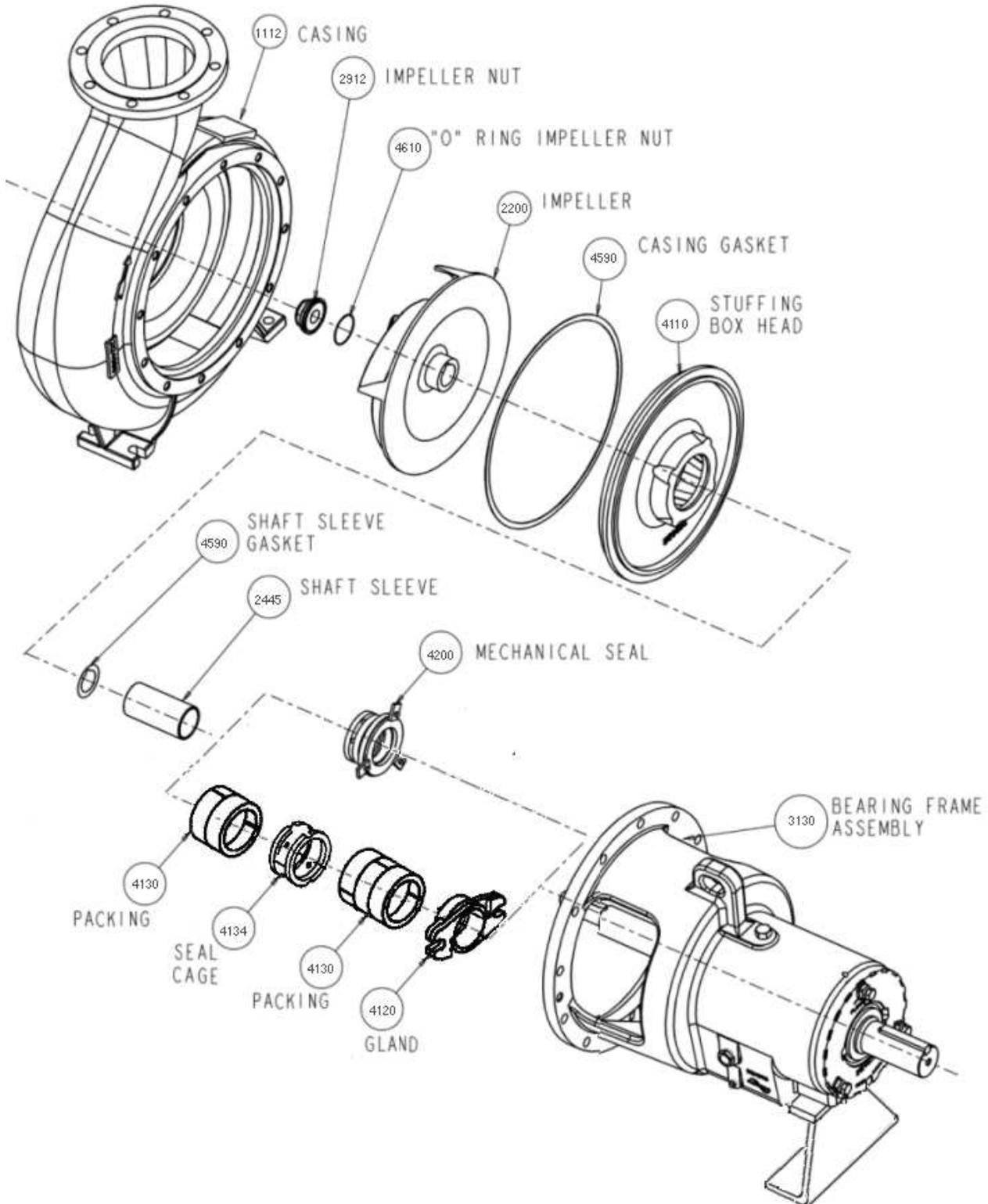
**8.3 Mark 3 Group 4 chemical pump frame exploded view**
