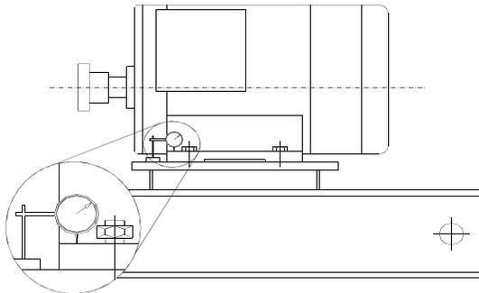
This is a check to ensure that there is no undue stress on the driver holding down bolts; due to non-level baseplate or twisting. To check, remove all shims and clean surfaces and tighten down driver to the baseplate. Set a dial indicator as shown in sketch and loosen off the holding down bolt while noting any deflection reading on the dial test Indicator - a maximum of 0.05 mm (0.002 in.) is considered
