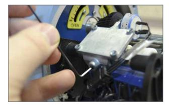
\*Potentiometer terminals may not be accessible if the AID CPT option is also fitted. In this instance it is important to ensure the POT does not slip throughout full valve travel. Current should change through 4-20 mA however tuning may be required. Refer to the next page for tuning instructions.
