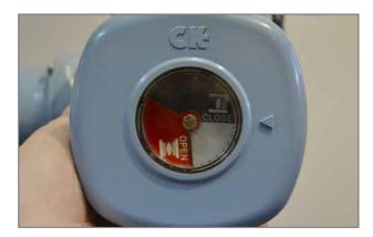
6) Move the actuator to the OPEN limit using electrical or operation or the handwheel.
