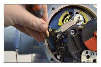
A 5mm Allen (Hex.) key and 0.8 x 4mm flat screwdriver with at least 120mm shaft length are required to perform commissioning of the CK Mechanical Switch Mechanism. A small torch may be required in environments with low level lighting.
