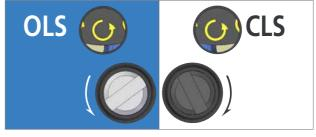
Rotate the OLS/CLS Adjustment Shaft Anti-Clockwise.
