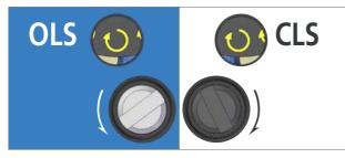
Rotate the OLS/CLS Adjustment Shaft Clockwise.
