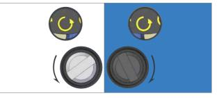
Rotate the OLS/CLS Adjustment Shaft Anti-Clockwise.
