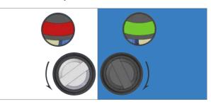
The limit switching point is near or made.
