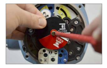
5) Confirm the CLOSE label is aligned correctly with the cover indication arrow.
