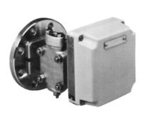
The PREX3000 instruments are pneumatic type transmitters which employ a combination of vector balance mechanism and involute mechanism. The instruments are featured by high resistance against adverse environments, high turn-down ratio, high accuracy, and ease of maintenance.
