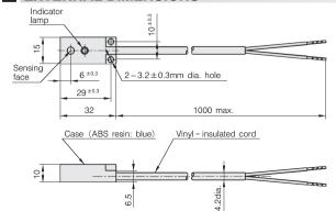
Vinyl-insulated cord (oil-resistant, bend-resistant type: 0.3mm², 60/0.08 dia., 2-core) 4.2mm dia
