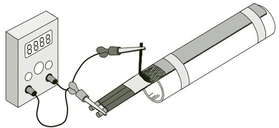
Connect the positive lead of the megger to the cable bus wires and the negative lead to the metallic braid.
