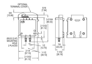
The Series 616KD One-Touch<sup>®</sup> Differential Pressure Transmitter senses the pressure of air and compatible gases and sends a standard 4 to 20 mA or optional voltage output signal. A wide range of models are available factory calibrated to specific ranges. A single push button properly adjusts both zero and span. New enclosure enables the 616KD to be mounted on a 35 mm DIN rail either via its side or back DIN rail clips.
