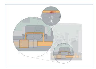
The mass flow sensor operates according to a thermal principle which has the advantage of providing the mass flow which is independent on pressure and temperature.
