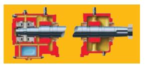
Split Sleeve Radial and Tilting Pad Thrust
