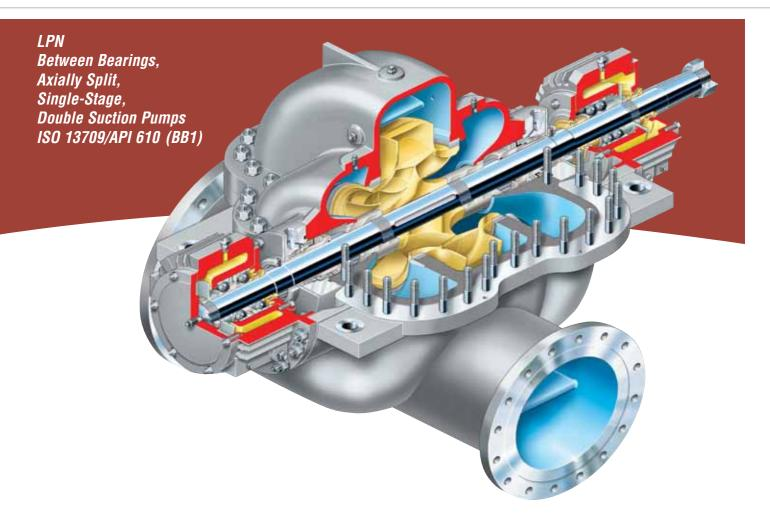
The Flowserve LPN is an axially split, single-stage pump designed to ISO 13709/API 610 (BB1), latest edition. With a double-suction impeller, the LPN is a natural solution for many low NPSH applications, such as those found in water and hydrocarbon transfer service.
