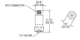
The MODEL VBT-1 Vibration Transmitter continuously detects the vibration in a system and monitors for unusual operating conditions and potential failure. The vibration is converted into an analog signal at the current output. The 2-wire loop power operation, combined with standard M12 micro cable connector and interchangeable mounting studs, make for a fast and reliable installation.
