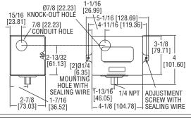
Reliable and convenient, SERIES AP pressure switch is a compact switch Reliable and convenient, series AP pressure switch is a compact for instrument air or other low pressure applications. Visible set point and external adjustment add convenience. Used on air, non-corrosive gas or liquid service compatible with wetted parts. Units are available in weather-proof and explosion-proof housing.
