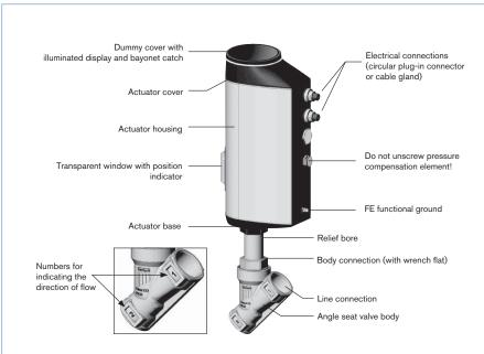
Structure, electromotive angle seat shut-off valve, Type 3320
