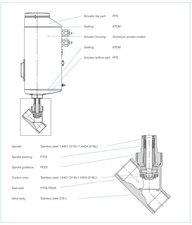
Note: The angle-seat shut-off valve **Type 3320** could be delivered with miscellaneous port connection (thread, weld ends and clamp), there are not represented in the picture, but are made with same material as the valve body.
