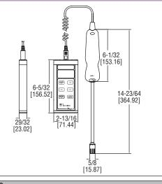
The **MODEL 485B** Thermo-Hygrometer is a versatile, compact, handheld instrument for measuring percentage of relative humidity and temperature in °F or °C. Dew point and wet bulb temperatures are derived from the relative humidity and temperature measurements and are displayed on the LCD.
