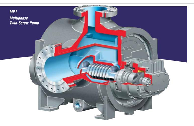
The Flowserve MP1 is the most robust twin-screw pump in the oil and gas industry. Engineered for multiphase pumping, it features a double-suction, timed twin-screw configuration built in accordance with API 676, latest edition. The design of the MP1 was further refined to provide the highest overall efficiency and lowest operating vibration levels of any multiphase, twin-screw pump.
