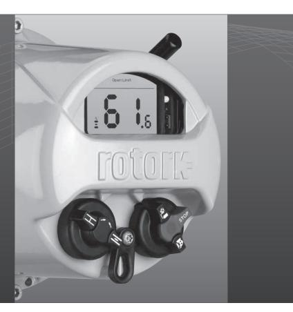
Rotork's proven IQ range of actuators now includes absolute position measurement, large information rich display, enhanced data logging, status and asset management plus additional control and indication features and options. IQ range actuators are self-contained, non-intrusive units for local and remote electrical operation of valves.
