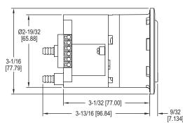
The Series MP Mini-Photohelic® Differential Pressure Switch/Gage combines the time proven Minihelic® II differential pressure gage with two SPDT switching setpoints. The Mini-Photohelic® is designed to measure and control positive, negative, or differential pressures consisting of non-combustible and non-corrosive gases. Gage reading is independent of switch operation. Switching status is visible by LED indicators located on the front and rear of the gage.
