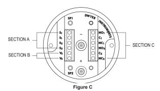
**Section A** contains external connections to the holding circuit for manual reset applications. The function and use of these connections varies somewhat depending on the circuit style of the instrument. See steps 7 and 9 for details.
