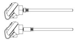
Style 81F - Secondary tube with slip flange mounting
