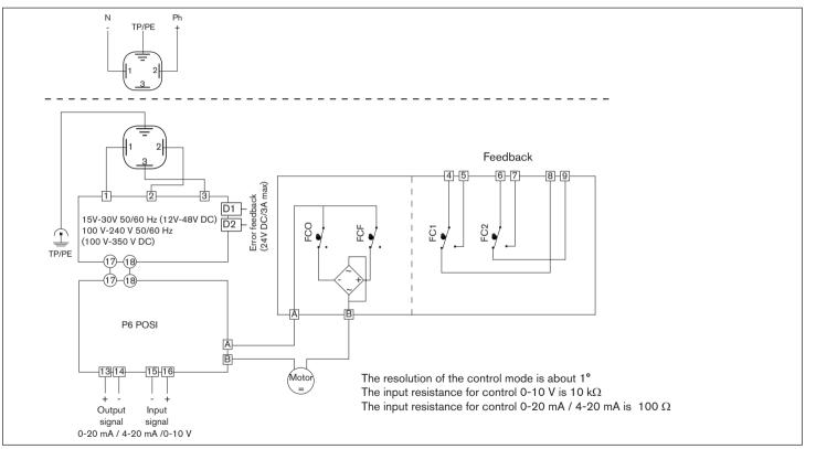
Fig. 3: Version with analog signal input
