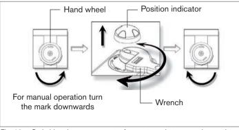
Fig. 12: Switching the rotary actuator from automatic to manual operation
