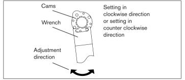
Fia. 5: Setting limit switches in counter clockwise and clockwise directions
