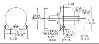
The SERIES 123 & 125 Boiler Water Level Controls are designed for boiler applications, the Model 123 is primarily used for low water cut-off or feed-water control. The 125 offers the same long lasting service with a direct action mercury switch movement that provides a close deadband where needed.
