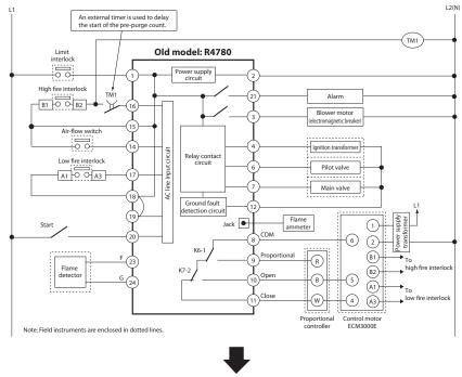
Three-minute pre-purge timer models are available for the BC-R35. So, unlike the R4780, the BC-R35 does not need an external timer.
