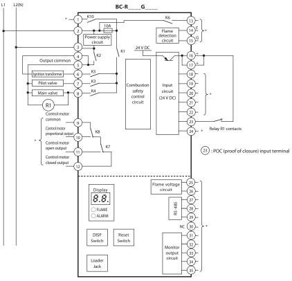
\* For connections of these terminals, follow the wiring instructions for the BC-R15/25/35.
