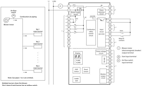
A BC-R controller is required for each burner.
