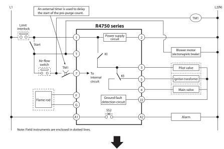
Three-minute pre-purge timer models are available for the BC-R25. So, unlike the R4750B, the BC-R25 does not need an external timer.
