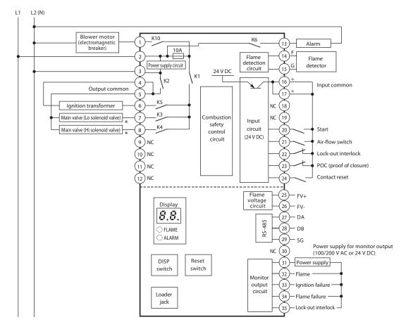
\* Content in () describes the situation when three-position (Off-Lo-Hi) control is used. If other than three-position control is used, connect to main valve (terminal 7).
