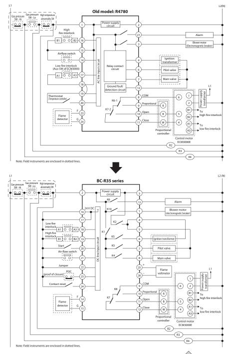
Since the interlock input of the BC-R15/25/35 detects failures using pulse signals, if relays are directly connected to the input, it will not work.
