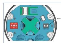
büS service interface Connection for CAN adapter or USB-büS interface set
