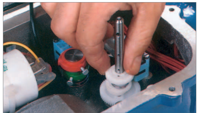
Auxilliary limit switch setting
