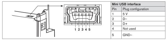
Figure 3: Mini USB interface configuration; for factory service
