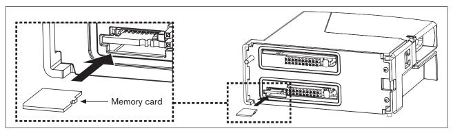
Figure 14: Replacing the micro SD card; controller module Type ME25
