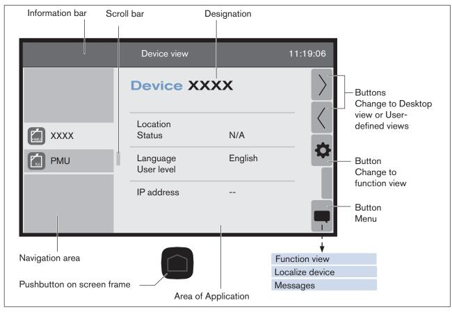
Figure 6: Device view of controller module (example)
