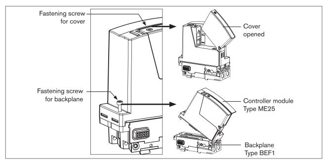
Figure 13: Replacing the device; controller module Type ME25
