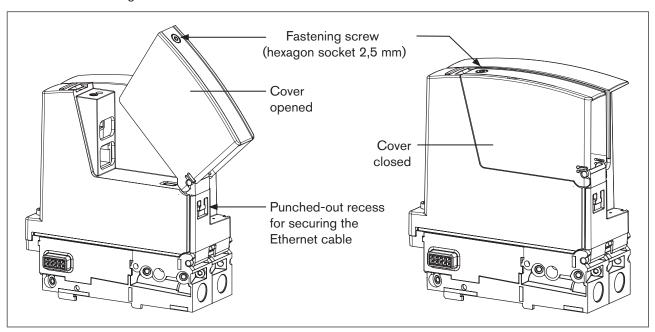
Figure 5: Access to interfaces USB and RJ45
