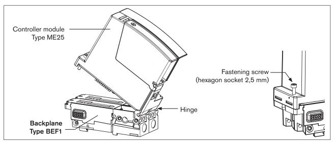
Figure 4: Mount controller module Type ME25 on backplane Type BEF1
