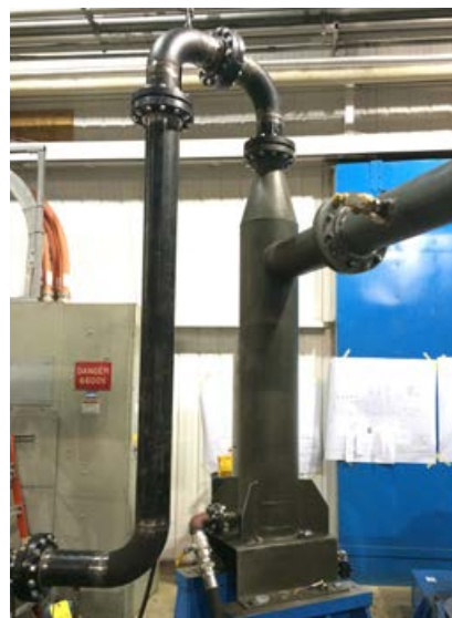
Liquid separator used to maintain stable temperatures in MP1 units running in high-GVF applications or as wet gas compressors
