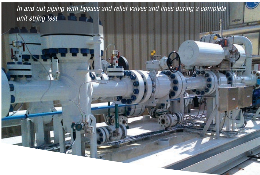
Fully compliant API Plan 53B systems to support robust multiphase mechanical seals mounted on a dedicated skid
