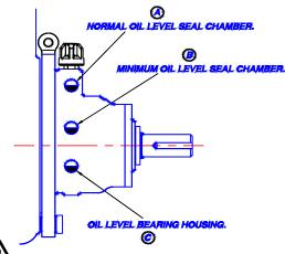
Always use the recommended Type and grade of oil, Mobil DTE Medium or Castrol Hyspin AWS 46. Never mix oil types.
