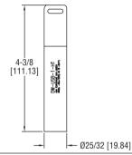
The MODEL DW-USB-1-HT High Temperature USB Data Logger allows users to monitor temperatures up to 257°F (125°C). The rigid, stainless steel enclosure protects the sensor against corrosion, impact, and water ingress.
