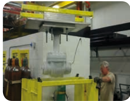
6" McCANNA cryogenic valve removed from -320 °F LN2 tank
