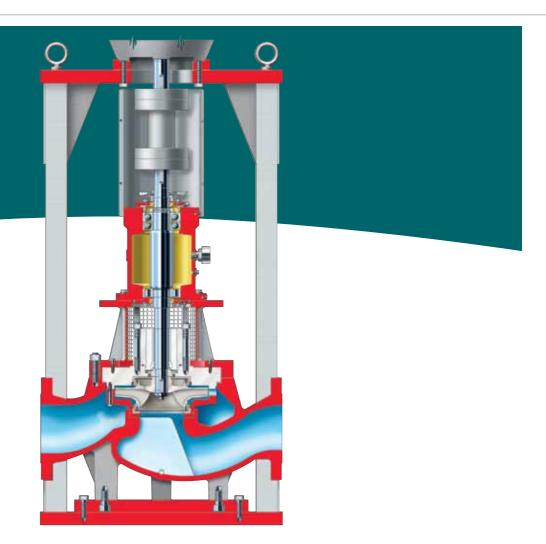
The PVXM meets and exceeds the rigorous requirements of API 610 / ISO 13709, latest edition, type OH3: mechanically sealed, flexibly coupled, vertical in-line pumps with a bearing frame. The PVXM design permits customized hydraulics for lowest total cost of ownership based upon:
