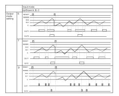
Output Modes S, T, and D can only be used with up/down counting inputs.
