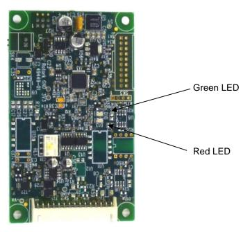
Figure 3: Field Unit Indication LEDs
