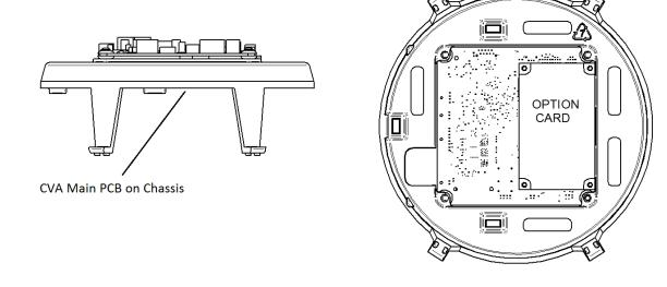
Figure 5: The FCU located on the underside of the control PCB in a CVA actuator
