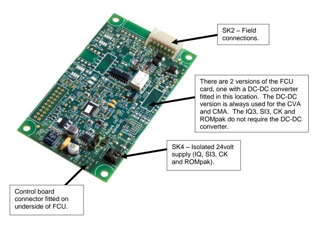
Figure 2: The IQ Pakscan Field Unit
