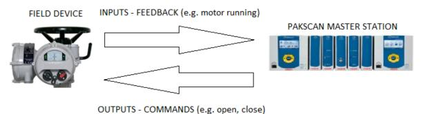
Figure 12: Input and Output Data Directions
