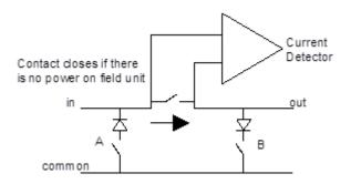
Figure 11: Loop Bypass relay
