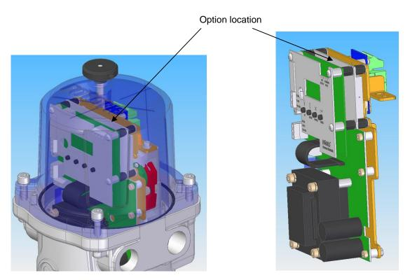
Figure 7: The FCU located in a CMA actuator
