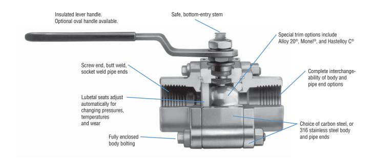
Flowserve Worcester Controls has tailored the LTS4 Series valves to meet the severe condition of Oil and Gas Production in Northern Climates. All materials and seals were carefully chosen to meet or exceed the -50°F (-45°C) minimum design temperature. Additionally, the LTS4 valve incorporates Worcester's standard three-piece design and components making the valve easy to service with readily available repair parts.
