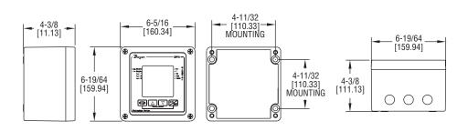
The SERIES DPM Particulate Monitor and Series PMS Particulate Sensor combine to provide a basic baghouse and cartridge filter leak detector designed for general maintenance planning and process protection. Leakage is gauged in real-time, on-thespot, without prior baseline data and without signal tuning and displayed on the digital readout in a bar graph and an absolute digital readout. An alarm point can be set by simply moving an indicator up and down the gauge with the key pad.
