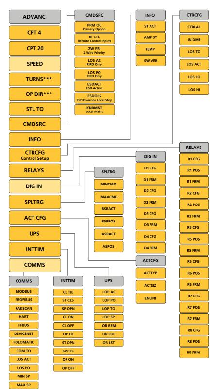
NOTE: Additional Relay, Digital Inputs and Comms menus shown are dependant on options fitted. Menus will not appear unless option is fitted.
