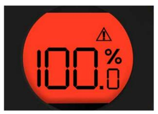
Fig 5.7 Actuator flashes Red and White alternatively when power failure occurs
