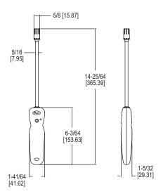
The Model RP2 Wireless Thermo-Hygrometer Probe for UHH/UHH2 measures relative humidity, temperature, dew point, and wet bulb temperatures when combined with Models UHH and UHH2 or the Dwyer Mobile Meter® app. In order to protect the sensor in higher air flow ducts, each probe comes with a membrane filter. Factory calibrated replacement humidity sensors can plug directly into the probe without requiring additional calibration.
